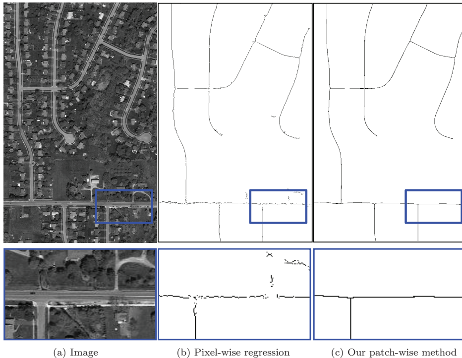
Figure 6.1: Limitation of pixel-wise approaches. Pixel-wise classifiers and regressors reach state-of-the-art performance in several Computer Vision tasks. However, the response of such methods does not take into account the very particular structure and the spatial relation present in the ground truth images. (a) An aerial road image. For this problem the ground truth is composed by a continuous 1-D curve. (b) Output of our method of Chap. 5. Since this method is based on pixel-wise regression, its output has discontinuities on the centerlines and isolated responses on the background. (c) The output of our method is obtained by projecting the patches of the score image of (b) into the closest ground truth patches from the training images. In this way the structure of the ground truth patches is transferred to the score image, resulting in a provably correct global spatial structure.
