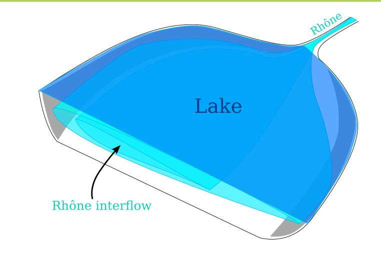
Numerical simulations using MITgcm code, finite volume approach, "classical" z vertical coordinate (Marshall et al., 1997), 35 levels with thickness increasing with depth (0.5 m at the surface). Horizontal quasi-orthogonal curvilinear grid with a resolution of approximately 200 m. Realistic surface forcing is derived from COSMO/MeteoSwiss simulations. The configuration limits numerical diffusion, following Hill et al. (2012).
