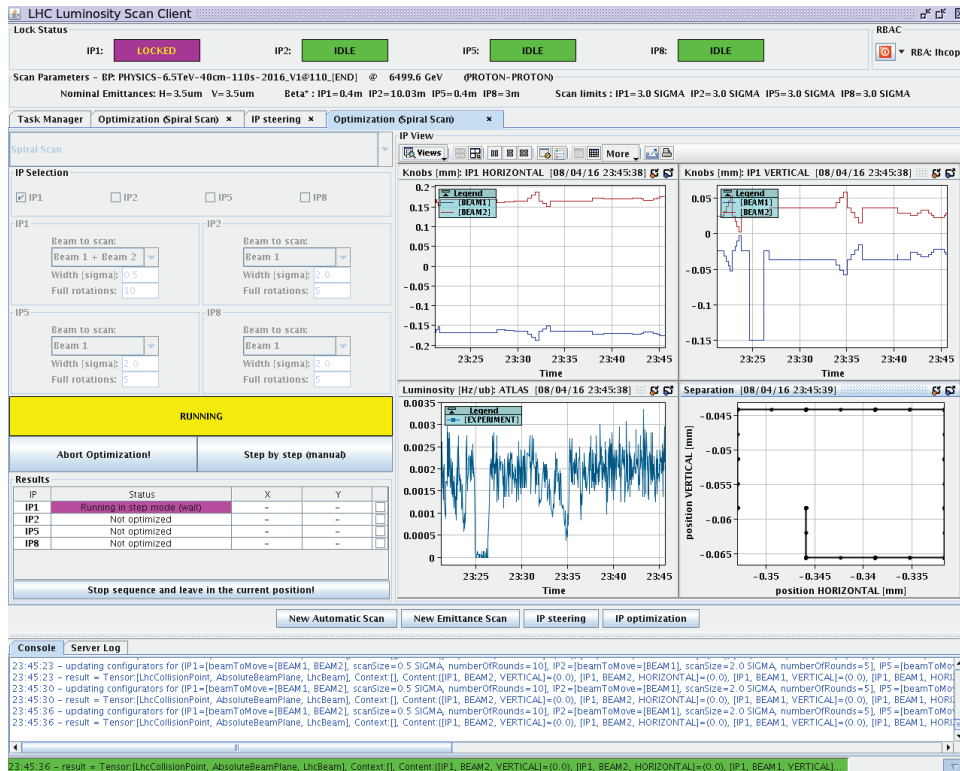
Figure C.6 – Finding collisions with a spiral scan (seen as a black line in the right bottom part, here in "rectangular form") on April 8 th 2016 when establishing first collisions after the winter stop in 2015/2016.
