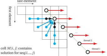
Figure 7.12 – Threads progress jointly along matrix diagonal. Dependencies can be reduced to immediately preceding matrix cells.
