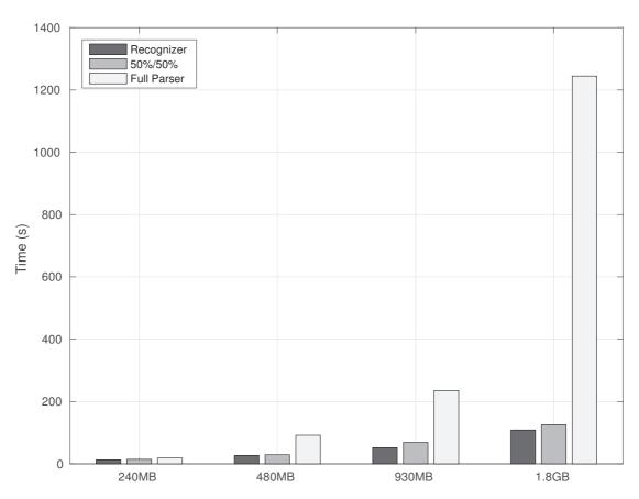
Figure 8.16 – Running time as we vary the file size from 240 to 1800 MB.
