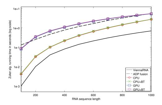
Figure 7.16 – Zuker algorithm running time
