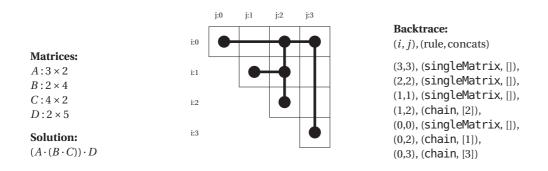
Figure 7.13 - A backtrace for an instance of the matrix multiplication problem
