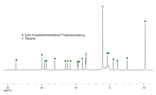
Figure A3:  $^{1}$ H NMR spectrum (200 MHz, tol-d<sub>8</sub>, 298K) of [U(9,10- phenanthrenediol) ( $^{Me}$ naphtquinolen)<sub>2</sub>] 3.
