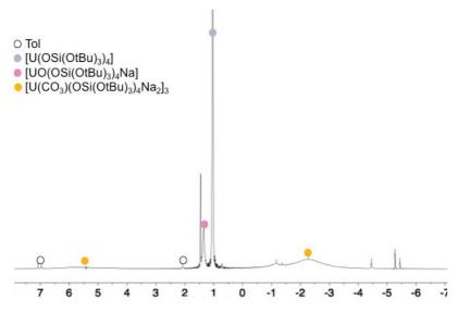
Figure III-28:  $^{1}$ H NMR spectrum (400MHz, tol-d<sub>8</sub>, 298K) of the crude mixture after addition of 1eq of  $CO_2$  to  $[U(OSi(OtBu)_3)_4Na]$
