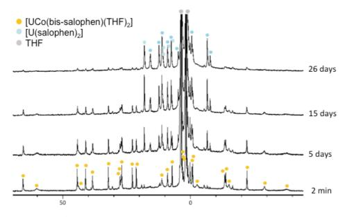
Figure II-10: <sup>1</sup>H NMR spectrum (200MHz, THF-d<sub>8</sub>, 298K) of complex 5, and evolution over time.
