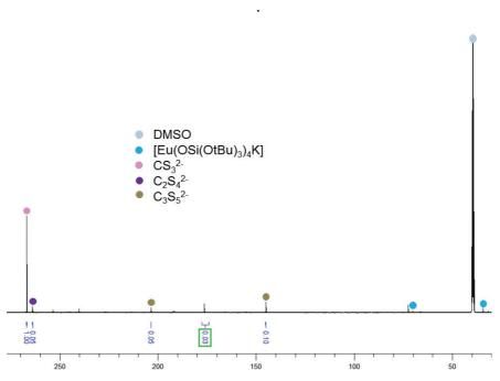
$Figure\ A34:\ Quantitative\ ^{13}C\ NMR\ spectrum\ (100MHz,\ DMSO-d_6,\ 298K)\ of\ the\ crude\ mixture\ reaction\ after\ the\ addition\ of\ 1eq\ of\ ^{13}CS_2\ to\ [Eu(OSi(OtBu)_3)_4K_2]\ 33-Eu\ after\ the\ removal\ of\ THF.$
