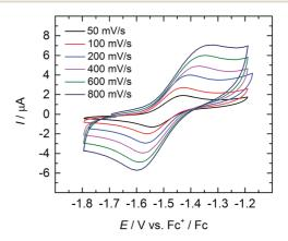
Fig. 5 Quasi-reversible oxidation wave of **3** at different scan rates. Measurement conducted in THF with  $\sim$ 0.1 M [N(n-Bu)<sub>4</sub>][BPh<sub>4</sub>] electrolyte, using Fc<sup>+</sup>/Fc couple as internal standard.
