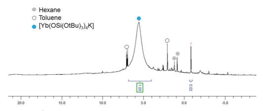
$Figure\ A36:\ In\ situ\ ^1H\ NMR\ spectrum\ (400\ MHz,\ tol-d_8,\ 298K)\ after\ addition\ of\ CO_2\ to\ [Yb(OSi(OtBu)_3)_4K_2]\ 33-Yb.$
