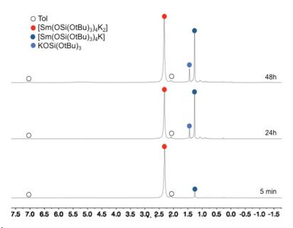
Figure IV-3: <sup>1</sup>H NMR spectrum (200MHz, tol-d<sub>8</sub>, 298K) of [Sm(OSi(OtBu)<sub>3</sub>)<sub>4</sub>K<sub>2</sub>], 33-Sm, and evolution over time.
