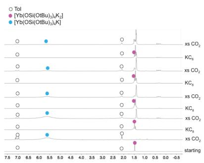
Figure IV-10: <sup>1</sup>H NMR spectra (200MHz, tol-d<sub>8</sub>, 298K) of the CO<sub>2</sub> reduction cycles.
