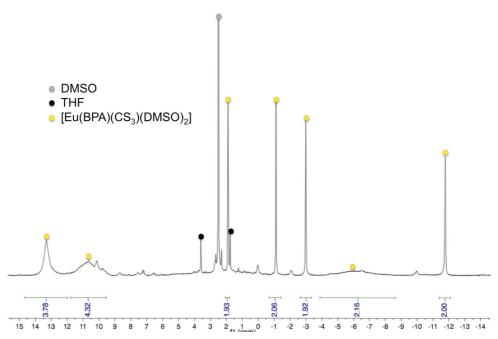
Figure A49:  $^{1}$ H NMR spectrum (400 MHz, DMSO-d<sub>6</sub>, 298K) of [Eu(BPA)(CS<sub>3</sub>)(DMSO)<sub>2</sub>] 44.
