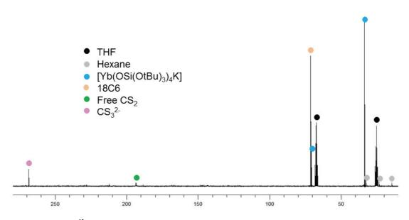
Figure A32: In situ  $^{13}$ C NMR spectrum (50 MHz, THF-d $_8$ , 298K) of the crude mixture reaction after the addition of 1eq of  $^{13}$ CS $_2$  to [Yb(OSi(OtBu) $_3$ ) $_4$ K $_2$ ] + 2eq 18C6.
