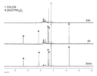
Figure IV-15:  $^{1}$ H NMR spectrum (400 MHz, CD<sub>3</sub>CN, 298K) of [Sm(TPA)<sub>2</sub>]I<sub>2</sub>, 38-Sm and evolution over time.
