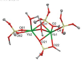
Figure IV-11: Solid state structure of one of the two complexes [Yb<sub>2</sub>(OSi(OtBu)<sub>3</sub>)<sub>4</sub>)(DME)], 35 (50% ellipsoids). Disorder and hydrogen atoms are omitted for clarity.
