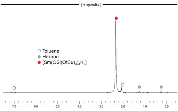
Figure A29:  $^1\text{H}$  NMR spectrum (400 MHz, tol-d\_8, 298K) of [Sm(OSi(OtBu)\_3)\_4K\_2] 33-Sm.
