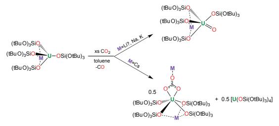
Scheme III-15: Addition of an excess of CO<sub>2</sub> to the [U(OSi(OtBu)<sub>3</sub>)<sub>4</sub>M] complexes (M=Li, Na, K, Cs).
