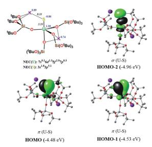
Fig. 7  $\,\sigma$  and  $\,\pi$  molecular orbitals ( $\alpha$ -spin) calculated for the monomer-1 using the small-core pseudopotential. The numbers in blue correspond to the natural charges and those in italics to the Wiberg bond orders. Hydrogen atoms are omitted for clarity.
