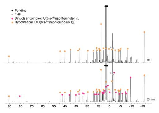
Figure II-6:  $^{1}$ H NMR spectra (200MHz, 298K) of the crude reaction between [U(bis- $^{Me}$ naphtquinolen)]2, 2 and 2eq of pyHCl in py-d5, after 30 min (bottom) and after 1 night (top).
