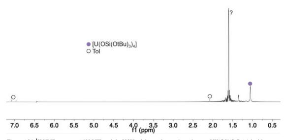
Figure A24:  $^1$ H NMR spectrum (400 MHz, tol-d<sub>8</sub>, 298K) of the crude reaction mixture of [U(OSi(OtBu)<sub>3</sub>)<sub>4</sub>] with excess N<sub>2</sub>O.
