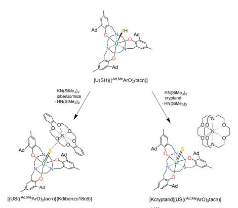
Scheme III-6: Synthesis of the terminal sulfide complexes [{US(( $^{Ad,Me}ArO$ )\_3tacn)}{Kdibenzo18c6}] and [Kcryptand][US(( $^{Ad,Me}ArO$ )\_3tacn)].
