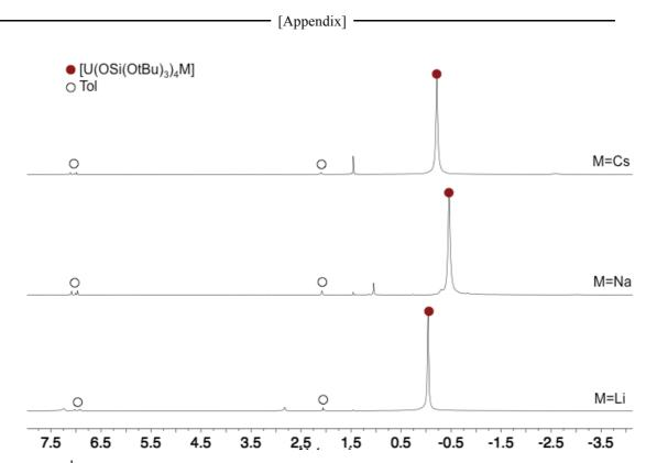
Figure A21:  $^{1}$ H NMR spectra (400 MHz, tol-d<sub>8</sub>, 298 K) of the [U(OSi(OtBu)<sub>3</sub>)<sub>4</sub>M] complexes M=Li 25 (bottom), M=Na 26 (middle), M=Cs 27 (top).
