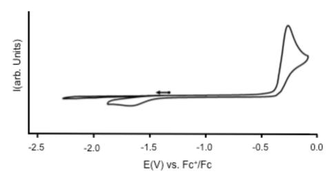
Figure A52: Cyclic voltammogram for K- $^{Me}$ naphtquinolen in ~0.1 M [Bu<sub>4</sub>N][PF<sub>6</sub>] pyridine solution at 100 mV.s<sup>-1</sup> scan-rate. No reduction event is observed when the voltammogram is swept initially from -1.4 V to the negative direction. An irreversible oxidation process attributed to the oxidation of the phenol moiety occurs at E = -0.26 V and is associated to the irreversible reduction occurring at -1.67 V.
