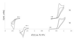
**Figure 8.** Cyclic voltammogram for 4 mm solutions of: a) [Eu(BPA) $_2$ ]OTf and b) [Yb(BPA) $_2$ ]OTf in  $\approx$  0.1 m [Bu $_4$ N][PF $_6$ ] acetonitrile solution at 100 mV s $^{-1}$
