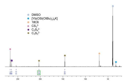
$Figure\ A33:\ Quantitative\ ^{13}C\ NMR\ spectrum\ (100MHz,\ DMSO-d_6,\ 298K)\ of\ the\ crude\ mixture\ reaction\ after\ the\ addition\ of\ 1eq\ of\ ^{13}CS_2\ to\ [Yb(OSi(OtBu)_3)_4K_2]\ +\ 2eq\ 18C6\ after\ the\ removal\ of\ THF.$
