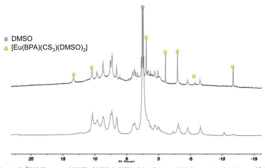
Figure A51:  $^{1}$ H NMR spectra (400 MHz, DMSO- $d_{6}$ , 298K) of the 1:2 (top) and 1:1 (bottom) reaction mixture of EuI $_{2}$  and KBPA after addition of 1eq of CS $_{2}$ .
