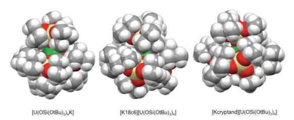
Figure III-18: Spacefilling representation of [U(OSi(OtBu)<sub>3</sub>)<sub>4</sub>K], [K18c6|[U(OSi(OtBu)<sub>3</sub>)<sub>4</sub>] and [Kcryptand][U(OSi(OtBu)<sub>3</sub>)<sub>4</sub>]. Solvent molecules and [K18c6]<sup>+</sup> and [Kcryptand]<sup>+</sup> cations are omitted for clarity.
