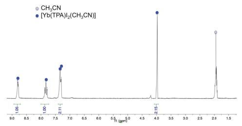
Figure A41:  $^{1}$ H NMR spectrum (200 MHz, CD<sub>3</sub>CN, 298K) of [Yb(TPA)I<sub>2</sub>(CH<sub>3</sub>CN)] 36.
