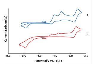
**Figure 4.** Cyclic voltammogram for 10 mM solutions of (a) **1-I** and (b) **2** in  $\sim$ 0.1 M [Bu<sub>4</sub>N][PF<sub>6</sub>] pyridine solution at 100 mV s<sup>-1</sup> scanrate.
