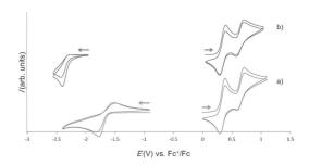
**Figure 9.** Cyclic voltammogram for 4 mm solutions of: a)  $[Eu(BPPA)_z]OTf$  and b)  $[Yb(BPPA)_z]OTf$  in  $\approx 0.1$  m  $[Bu_4N][PF_6]$  acetonitrile solution at 100 mV s<sup>-1</sup> scan rate.
