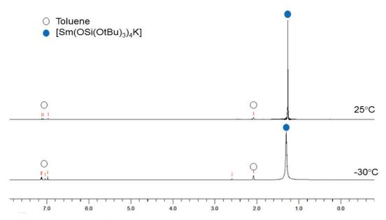
Figure A27:  $^1H$  NMR spectra (400 MHz, tol-d\_8) of [Sm(OSi(OtBu)\_3)\_4K] 32-Sm at -30°C (bottom) and 25°C (top).
