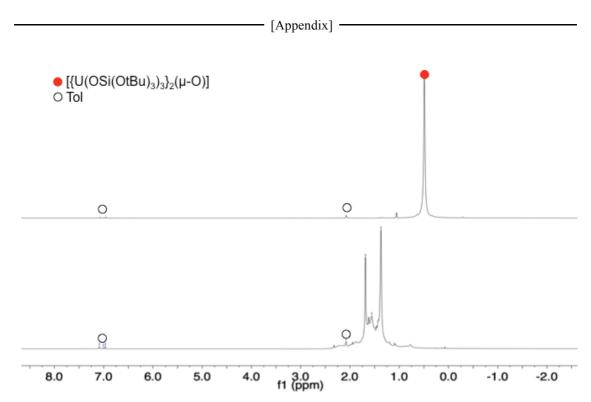
Figure A23:  $^1H$  NMR spectrum (400 MHz, tol-d\_8, 298K) of the crude reaction mixture of [U(OSi(OtBu)\_3)\_3]\_2 with excess N\_2O (bottom) and of [{U(OSi(OtBu)\_3)\_3}\_2(\mu-O)] 30 (top).
