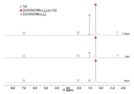
Figure III-32: <sup>1</sup>H NMR (400 MHz, tol-d<sub>8</sub>, 298K) spectrum of [{U(OSi(OtBu)<sub>3</sub>)<sub>3</sub>}<sub>2</sub>(µ-O)], 30 and evolution over time.
