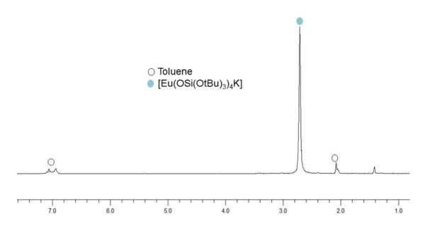
Figure A30:  $^1$ H NMR spectrum (200 MHz, tol-d<sub>8</sub>, 298K) of the supernatant of the reaction of [Eu(OSi(OtBu)<sub>3</sub>)<sub>4</sub>K<sub>2</sub>] 33-Eu with 1eq of PhNNPh.
