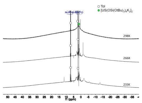
Figure III-12: Variable temperature <sup>1</sup>H NMR spectra (400 MHz, tol-d<sub>8</sub>) of [US(OSi(OtBu)<sub>3</sub>)<sub>4</sub>K<sub>2</sub>]<sub>2</sub>, 16.
