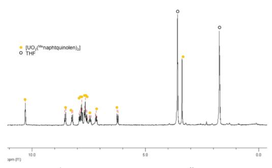
Figure A4:  $^1$ H NMR spectrum (200 MHz, THF-d $_8$ , 298K) of [UO $_2$ ( $^{Me}$ naphtquinolen) $_2$ ] 4.
