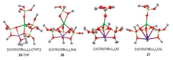
Figure III-26: Solid state structures of [U(OSi(OtBu)<sub>3</sub>)<sub>4</sub>M] complexes (M=Li 25, Na 26, K or Cs 27) (50% ellipsoids). Hydrogen atoms, methyl groups and lattice solvent molecules are omitted for clarity.
