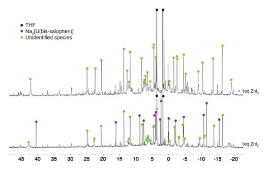
Figure II-12: <sup>1</sup>H NMR spectrum (200 MHz, THF-d<sub>8</sub>, 298 K) of the 1:1 reaction mixture of Na<sub>2</sub>[U(bis-salophen)] and ZnI<sub>2</sub> (bottom) and after another addition of ZnI<sub>2</sub> (top).
