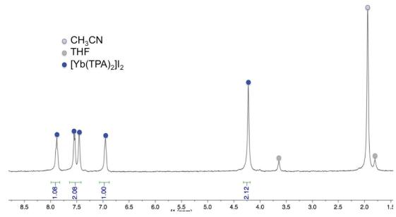
Figure A42:  $^{1}$ H NMR spectrum (200 MHz, CD<sub>3</sub>CN, 298K) of [Yb(TPA)<sub>2</sub>]I<sub>2</sub> 38-Yb.
