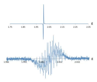
Figure IV-6: EPR spectra of solid KPhNNPh suspended in a toluene/hexane mixture (20/2) (top) and in DME/THF (100/1) solution (bottom) at 292K with 33dB of attenuation.
