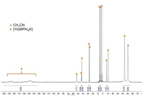
Figure A47: <sup>1</sup>H NMR spectrum (200 MHz, CD<sub>3</sub>CN, 298K) of [Yb(MPA)<sub>2</sub>K] 43.
