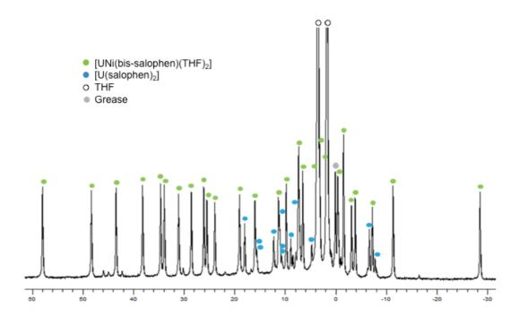
$Figure~A6: {}^{1}H~NMR~spectrum~(200~MHz, THF-d_{8}, 298~K)~of~the~1:1~crude~reaction~mixture~of~Na_{2}[U(bis-salophen)]\\ and~[NiI_{2}(THF)_{0.2}].$
