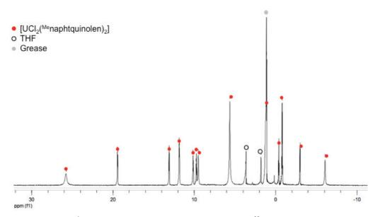
Figure A1:  $^{1}$ H NMR spectrum (200 MHz, THF-d $_{8}$ , 298) of [UCl $_{2}$ ( $^{Me}$ naphtquinolen) $_{2}$ ] 1-Cl.
