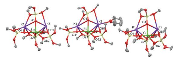
Figure IV-2: Solid state structure of  $[Ln(OSi(OtBu)_3)_4K_2]$  complexes, 33-Sm (left), 33-Eu.THF (middle), 33-Yb.tol (right) (50% ellipsoids). Methyl groups and solvent molecules are omitted for clarity.
