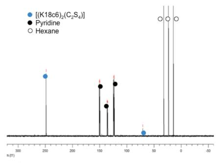
$Figure~A13: ^{13}C~NMR~spectrum~(100~MHz,~py-d_5,~298K)~of~the~crystals~of~[(K18c6)_2C_2S_4]. Py~isolated~from~pyridine/hexane.$
