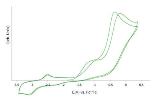
$Figure\ A54:\ Cyclic\ voltammograms\ of\ [US(OSi(OtBu)_3)_4K_2]_2,\ 16\ in\ \sim 0.1\ M\ [Bu_4N][PF_6]\ THF\ solution\ at\ 100\ mV.s^{-1}\ scan-rate$
