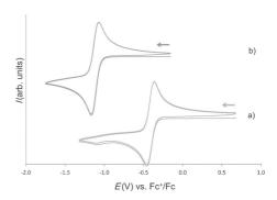
**Figure 7.** Cyclic voltammogram for 4 mm solutions of: a)  $[Eu(L1)_2]OTf$ ; b)  $[Yb(L1)_2]OTf$  in  $\approx 0.1$  m  $[Bu_4N][PF_6]$  acetonitrile solution at 100 mV s<sup>-1</sup> scan
