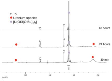
Figure III-3:  $^1H$  NMR spectrum (200MHz, tol-d $_8$ , 298K) of the crude reaction mixture of  $CS_2$  and  $[U(OSi(OtBu)_3)_4K]$  over the course of 2 days.
