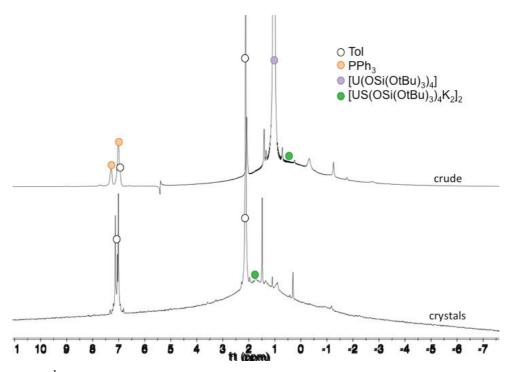
$Figure~A16:~^{1}H~NMR~spectrum~(200~MHz, tol-d_{8}, 298K)~of~the~1:0.5~reaction~mixture~of~[U(OSi(OtBu)_{3})_{4}K]~and~Ph_{3}PS~(top)~and~of~[US(OSi(OtBu)_{3})_{4}K_{2}]_{2}~16~(bottom).$
