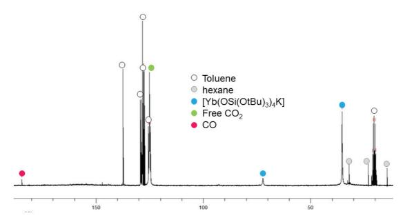
Figure A38:  $^{13}\mathrm{C}$  NMR spectrum (50MHz, tol-d\_8, 298K) of the crude mixture reduction of  $^{13}\mathrm{CO}_2$  by  $[Yb(OSi(OtBu)_3)_4K_2]$  33-Yb.
