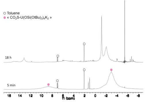
Figure A18:  $^1H$  NMR spectrum (400 MHz, tol-d<sub>8</sub>, 298 K) of the crude mixture after addition of an excess of  $^{13}CO_2$  to  $[US(OSi(OtBu)_3)_4K_2]_2$  16 after 5 min (bottom) and after 18 h (top).
