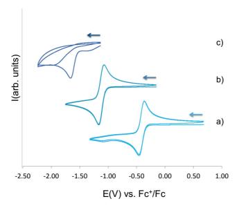
Figure IV-23: Cyclic voltammograms for 4 mM solutions of a)  $[Eu(TPA)_2]OTf_3$ , b)  $[Yb(TPA)_2]OTf_3$  and c)  $[Sm(TPA)_2]OTf_3$  in ~0.1 M  $[Bu_4N][PF_6]$  acetonitrile solution at 100 mV.s-1 scan-rate.
