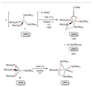
Scheme 2 Reaction of [K(18c6)][U(OSi(O $^t$ Bu) $_3$ ) $_4$ ], 1 (top) and of [U(OSi(O $^t$ Bu) $_3$ ) $_4$ K], 2 (bottom) with CO $_2$ .
