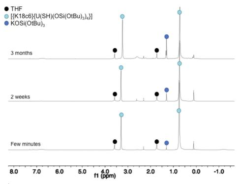
Figure A20:  $^1$ H NMR spectra (400 MHz, THF-d<sub>8</sub>, 298 K) of the stability follow up of [{K18c6}{U(SH)(OSi(OtBu)<sub>3</sub>)<sub>4</sub>}], 22, over time.
