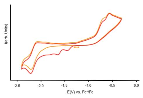
$\label{eq:figure A53: Cyclic voltammograms of [U(bis-$^{Me}$naphtquinolen)]_2, 2 in $\sim$0.1 M [Bu_4N][PF_6]$ pyridine solution at 100 mV.s -1 scan-rate. First scan: orange; second scan: red.}$
