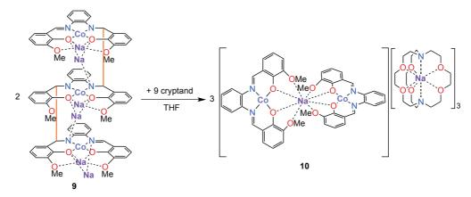
Scheme II-17: Synthesis of the Co(0) complex [Na(cryptand)]<sub>3</sub>[(Co(OMesalophen))<sub>2</sub>Na], 10.
