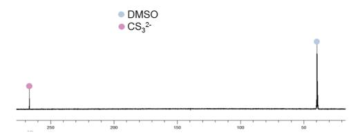
Figure A35:  $^{13}$ C NMR spectrum (100MHz, DMSO-d<sub>6</sub>, 298K) of the crystals of [(K<sub>2</sub>CS<sub>3</sub>)<sub>5</sub>(DMSO)<sub>12</sub>]<sub>n</sub>.
