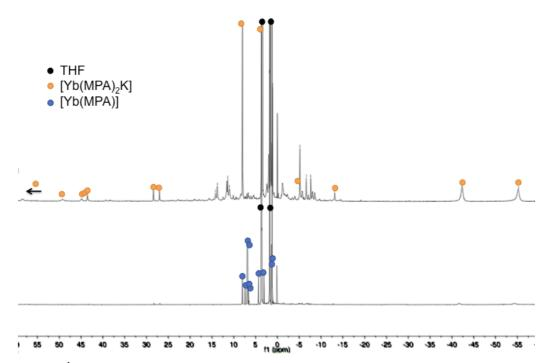
Figure IV-21:  $^1H$  NMR spectra (400 MHz, THF-d $_8$ , 298K) of the 1:2 (top) and 1:1 (bottom) YbI $_2$  and K $_2$ MPA reaction mixtures at -40°C in THF-d $_8$ .
