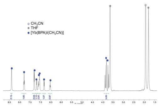
Figure A45: <sup>1</sup>H NMR spectrum (200 MHz, CD<sub>3</sub>CN, 298K) of the 1:1 reaction mixture of YbI<sub>2</sub> and KBPA.
