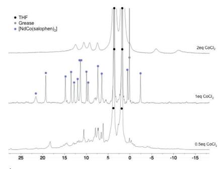
Figure II-14:  $^1$ H NMR spectra (200 MHz, THF-d<sub>8</sub>, 298 K) of the 1:0.5 (bottom), 1:1 (middle) and 1:2 (top) reaction mixtures of  $K_3[Nd(bis-salophen)]$  and  $CoCl_2$ .
