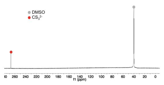
Figure A17:  $^{13}C$  NMR spectrum (100 MHz, DMSO-d<sub>6</sub>, 298K) of the 1:2 reaction mixture of complex [US(OSi(OtBu)\_3)\_4K\_2]\_2 16 and  $^{13}CS_2.$
