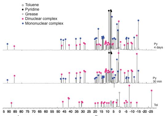
Figure II-3:  $^1H$  NMR spectra (200 MHz, 298K) of complex  $[U(bis^{-Me}naphtquinolen)]_2$ , 2, in tol-d<sub>8</sub> (bottom) and after dissolution of 2 in py-d<sub>5</sub>: after 30 min (middle), after 4 days (top).
