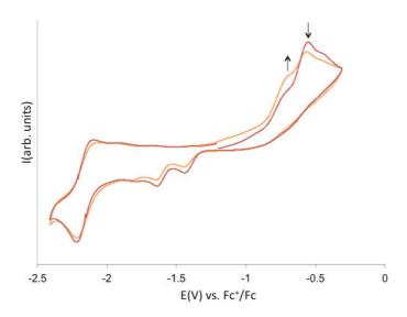
Figure II-5: Cyclic voltammograms of complex 2 in ~0.1 M [Bu<sub>4</sub>N][PF<sub>6</sub>] pyridine solution at 100 mV.s-1 scan-rate. Red curve: on a freshly prepared solution. Orange curve: on the same solution after 1 hour.
