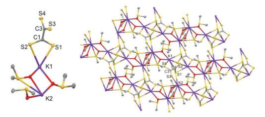
Figure III-6: Solid state structure of  $[K_2C_2S_4(DMSO)_3]_n$ , asymmetric unit (left) and 2D coordination polymer (right) (50% ellipsoids). Hydrogen atoms are omitted for clarity.
