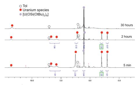
Figure III-2:  $^1H$  NMR spectrum (200MHz, tol-d<sub>8</sub>, 298K) of the crude reaction mixture of  $CS_2$  and  $[K18c6][U(OSi(OtBu)_3)_4]$  over the course of 2 days.
