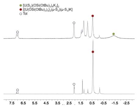
Figure A15: 1H NMR spectra (400 MHz, tol-d<sub>8</sub>, 298K) of the reaction mixture of [U(OSi(OtBu)<sub>3</sub>)<sub>4</sub>K] with 0.125eq (top) and 0.25eq (bottom) of  $S_8$ .
