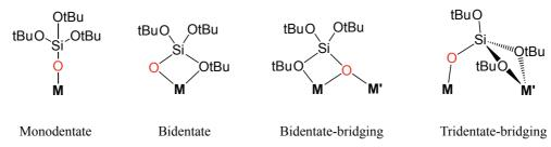
Figure III-1: Possible binding modes of the tris(tert-butoxy)siloxide ligand.
