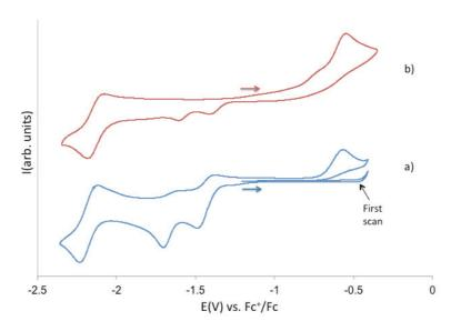
Figure II-4: Cyclic voltammograms for 10 mM solutions of a) complex 1-I and b) complex 2 in  $\sim$ 0.1 M [Bu<sub>4</sub>N][PF<sub>6</sub>] pyridine solution at 100 mV.s-1 scan-rate
