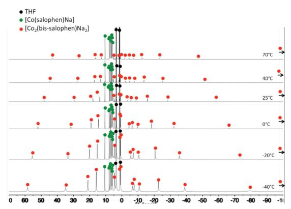
Figure A9: Variable temperature  $^1H$  NMR spectra (400 MHz, THF-d<sub>8</sub>) from -40°C to 70°C of a 0.353M solution of [Co(salophen)] reacted with one equivalent of Na.
