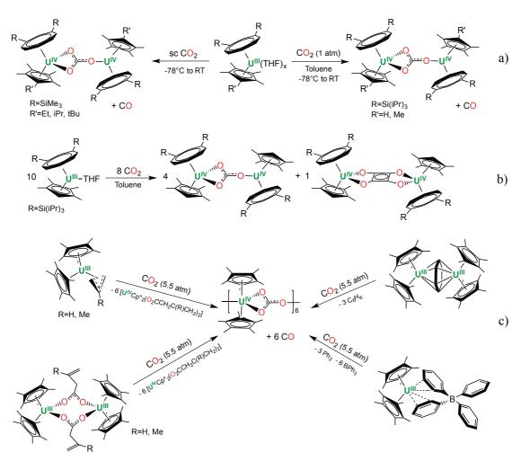
Scheme I-10: Reductive disproportionation of  $CO_2$  by organometallic the U(III) complexes: a)  $[U(COT^R)(Cp^{*R'})]$  with excess  $CO_2$ ,  $^{93}$  b)  $[U(COT^{Si(IPr)3})(Cp^{*H})]$  with 8eq of  $CO_2$ ,  $^{94}$  and c) syntheses of  $[UCp^*_2(\mu-CO_3)]_6$  from the reductive disproportionation of  $CO_2$  by different U(III) metallocenes.
