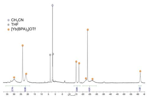
Figure A44: <sup>1</sup>H NMR spectrum (200 MHz, CD<sub>3</sub>CN, 298K) of the 1:2 reaction mixture of Yb(OTf)<sub>3</sub> and KBPA.
