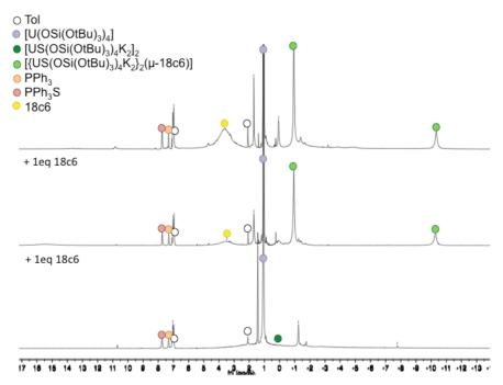
Figure III-14: <sup>1</sup>H NMR spectrum (400 MHz, tol-d<sub>8</sub>, 298 K) of the 1:1 reaction mixture of [U(OSi(OtBu)<sub>3</sub>)<sub>4</sub>K] and Ph<sub>3</sub>PS (bottom), after addition of 1eq of 18c6 per U to the crude mixture (middle) and after another addition of 1eq of 18c6 per U.
