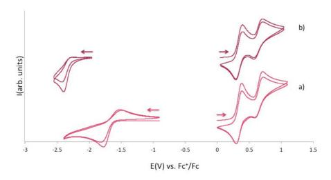
Figure IV-25: Cyclic voltammograms for 4 mM solutions of a)  $[Eu(BPPA)_2]OTf$  and b)  $[Yb(BPPA)_2]OTf$  in ~0.1 M  $[Bu_4N][PF_6]$  acetonitrile solution at 100 mV.s-1 scan-rate.
