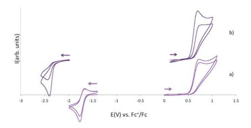
Figure IV-24: Cyclic voltammograms for 4 mM solutions of a)  $[Eu(BPA)_2]OTf$  and b)  $[Yb(BPA)_2]OTf$  in  $\sim 0.1$  M  $[Bu_4N][PF_6]$  acetonitrile solution at 100 mV.s-1 scan-rate.
