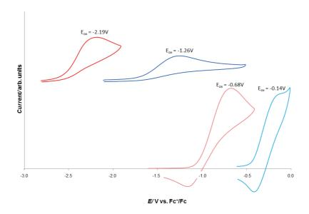
Figure IV-4: Cyclic voltammogram for  $EuI_2$  (light blue),  $YbI_2$  (light red), 33-Eu + 2eq 18C6 (blue) and 33-Yb + 2eq 18C6 (red) recorded at 6mM concentration in ~0.1 M [Bu<sub>4</sub>N][PF<sub>6</sub>] THF solution at 100 mV.s<sup>-1</sup> scan-rate with a glassy carbon working electrode.
