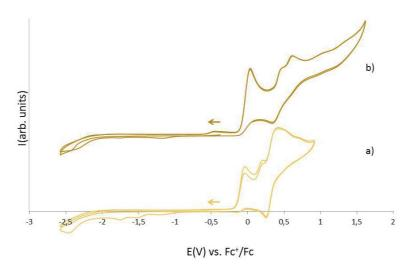
Figure IV-26: Cyclic voltammograms for 4 mM solutions of a) [Eu(MPA)<sub>2</sub>K] and b) [Yb(MPA)<sub>2</sub>K] in ~0.1 M [Bu<sub>4</sub>N][PF<sub>6</sub>] acetonitrile solution at 100 mV.s-1 scan-rate.
