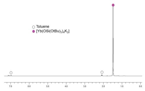
Figure A28:  $^1$ H NMR spectrum (400 MHz, tol-d<sub>8</sub>, 298K) of [Yb(OSi(OtBu)<sub>3</sub>)<sub>4</sub>K<sub>2</sub>] 33-Yb.
