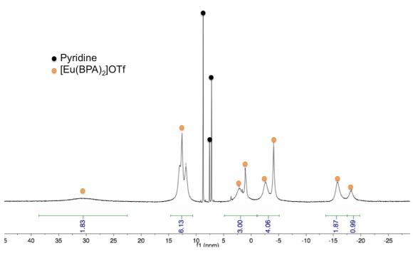
Figure A43:  $^1H$  NMR spectrum (200 MHz, py-d5, 298K) of  $[Eu(BPA)_2]OTf\,39.$
