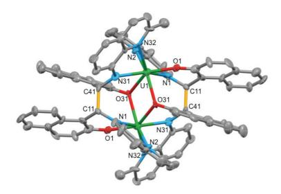
Figure II-2: Solid state structure of [U(bis-Menaphtquinolen)]<sub>2</sub>.(tol)<sub>2</sub>, 2.(tol)<sub>2</sub> (50% ellipsoids). The C-C bonds formed by the reduction of the imino functions are represented in orange. Hydrogen atoms and solvent molecules are omitted for clarity.
