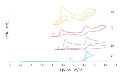
Figure IV-22: Cyclic voltammograms of TPA (4mM) (a), KBPA (<4mM) (b), KBPPA (4mM) (c) and  $K_2$ MPA (4mM) (d) in ~0.1 M [Bu<sub>4</sub>N][PF<sub>6</sub>] acetonitrile solution at 100 mV.s-1 scan-rate.
