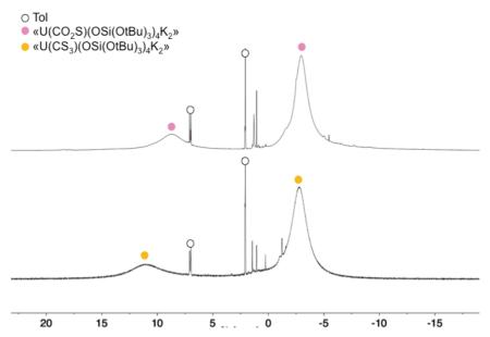
Figure III-19:  $^1H$  NMR spectra (400MHz, tol-d<sub>8</sub>, 298K) of the crude mixture right after addition of 1eq of  $^{13}CS_2$  per U atom to 16 (bottom) and after addition of an excess of  $^{13}CO_2$  to 16.
