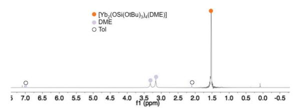
Figure A40:  $^1$ H NMR spectrum (200MHz, tol-d\_8, 298K) of the 1:2 reaction mixture of [Yb(HMDS)\_2] and HOSi(OtBu)\_3.
