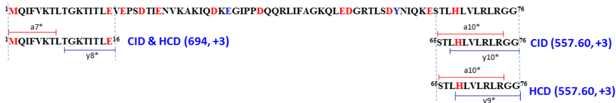
Figure 5.19 MS/MS of metallated fragments of RAPTA-T: Ubiquitin incubations digested with GluC. Full length ubiquitin sequence with probable binding sites in red and inaccessible binding sites in blue is shown above. Each metallated digest parent ion chosen for MS/MS is displayed with fragmentation type, mass and charge state. Relevant metallated MS/MS daughter ions obtained are displayed as N-terminal ions top, C-terminal ions bottom and internal ions highlighted green on the parent ion sequence.
