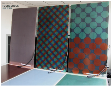
Figure 1.5-5: BIPV module with digital prints on the front glazing by CC EASE, HSLU. Photo credit: Stephen Wittkopf.
