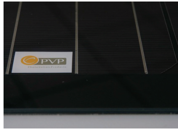
Figure 5.4-5: Comparison between the wafer and backsheet colour of PV sample 2.
