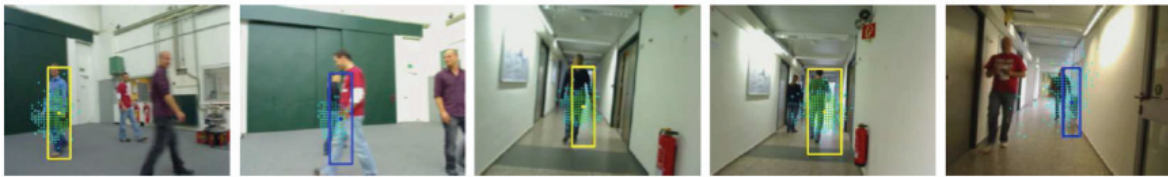
Figure 3.5-6. A demonstration of person tracking. Green points mark the regions that match with the target, while cyan points mark regions that don't. Yellow rectangle means that more than 30% of the region matches with the target, otherwise the object is framed with a blue rectangle. Source: [151] with permission of Springer.
