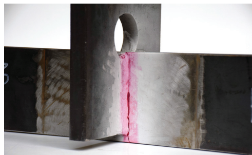
Figure 3.11 – Overall view of a failed specimen under proportional load
