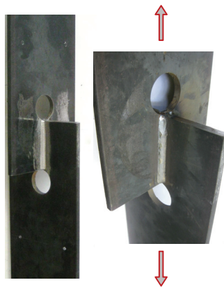
Figure 3.8 – “Proof of concept” shear test on slotted hole plate
