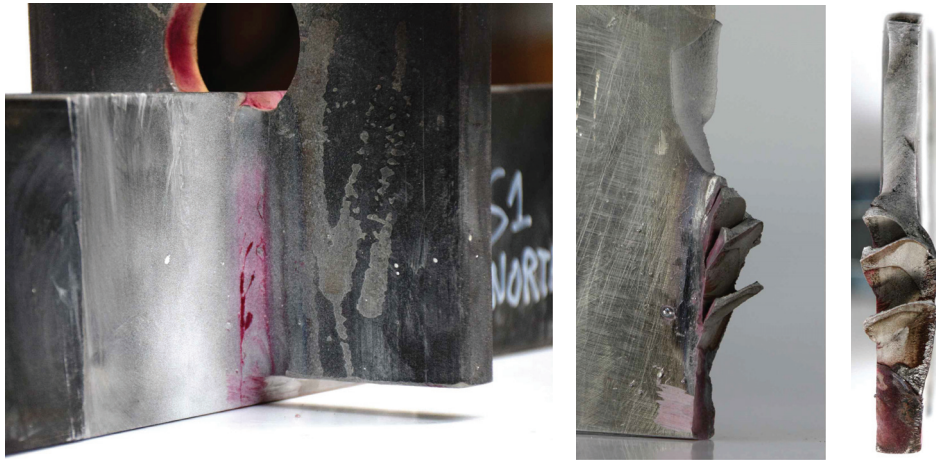
Figure 3.9 – Typical crack pattern for tests under uniaxial shear stress
