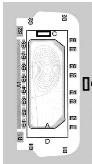
Figure 2. A poloidal cross-section of TCV showing the single (A and D) and multi (B and C) turn loops used for diamagnetic measurements. The ohmic transformer coils A1, B1, B2, C1, C2, D1 and D2 and the poloidal field shaping coils E1–E8 and F1–F8.
