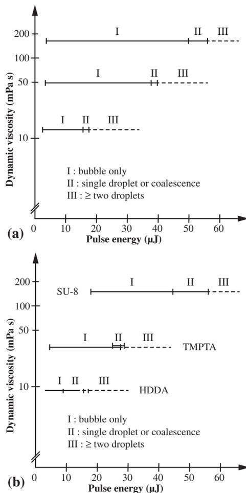
FIG. 3. Jetting regimes of inks with various dynamic viscosities for the same capillary diameter ( $300\ \mu\text{m}$ ). The y axis has a logarithmic scale, and the distance  $Z$  between the laser focal spot and meniscus is kept constant at  $500\ \mu\text{m}$ . (a) Newtonian water-glycerol solutions. (b) Non-Newtonian polymer solutions.
