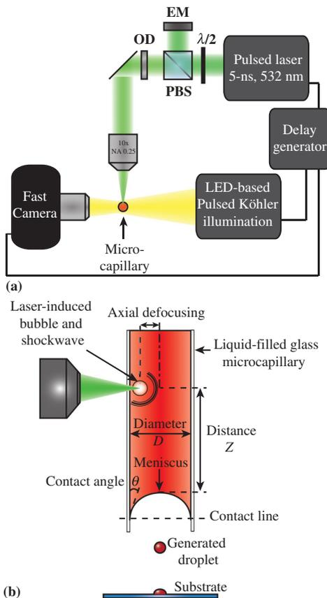
FIG. 1. Experimental setup. (a) Top view of the time-resolved imaging setup; the capillary axis is perpendicular to the graph.  $\lambda/2$ , half-wave plate; PBS, polarizing beam splitter; EM, energy meter; OD, optical density. (b) Side view of the microcapillary in which the droplets are generated and a description of the experimental parameters impacting the droplet size and velocity.
