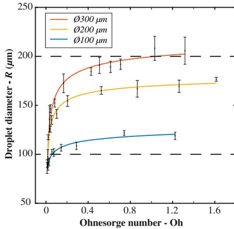
FIG. 5. Satellite-free drop diameter of water-glycerol mixtures as a function of the Ohnesorge number for different capillary sizes. The distance  $Z$  between the laser focal spot and the meniscus is kept constant at  $Z = 500, 400,$  and  $350 \mu\text{m}$ , respectively, for  $D = 300, 200,$  and  $100 \mu\text{m}$ . Power-law fits are also displayed. Each data point is the results of at least ten experiments.
