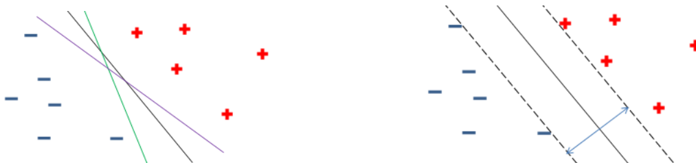
Figure 10 : Illustration of a 2D feature space, with objects of the positive class and negative class, depicted as red + and blue – respectively. Several lines can separate the two classes (left) but the best solution is the line that results in the maximal margin (right).
