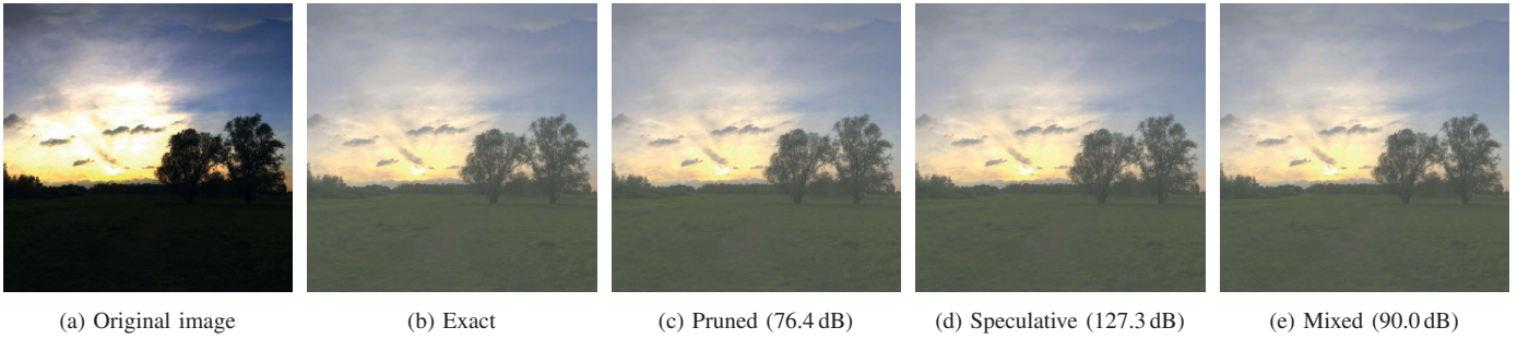
Fig. 6: Original image (a) and tone-mapped images obtained by each of the 4 cores (b-e). PSNR is indicated for images processed by the approximate FPUs. Image size is 512 \times 512 pixels.
