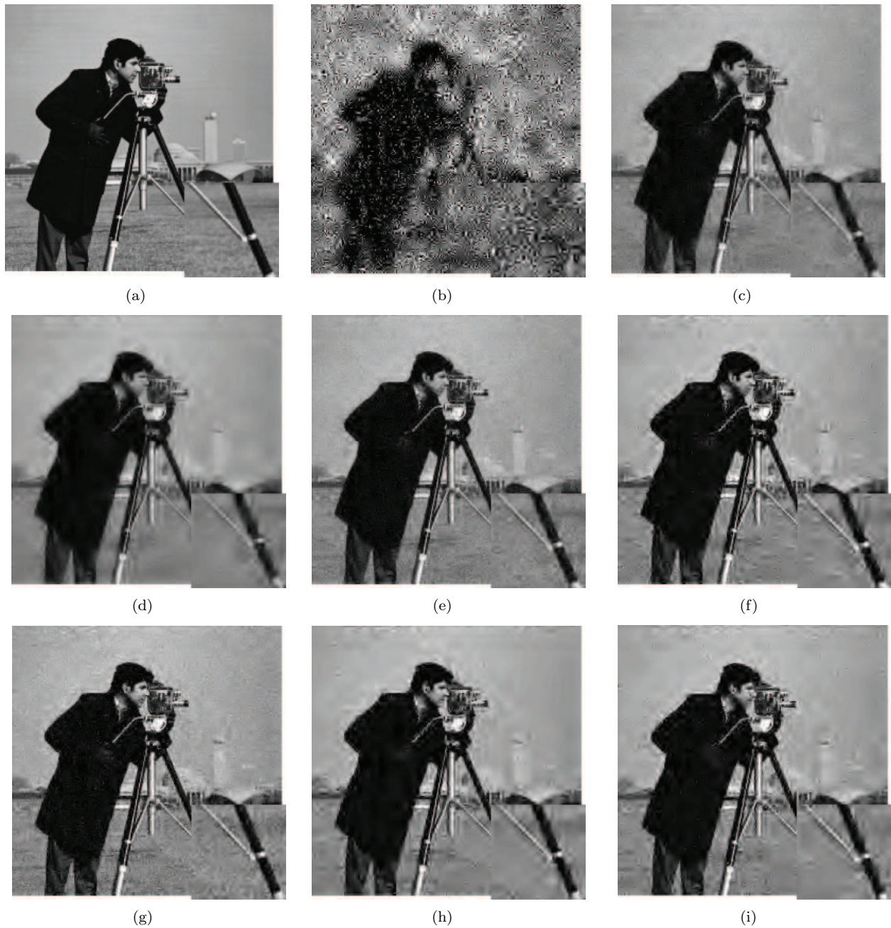
Figure 6 Cameraman image reconstruction (with zoomed of the bottom right area) example from Cauchy corrupted measurements. (a) Original image. (b) Reconstructed image using \ell_1 -LS (SER=7.3 dB). (c) Reconstructed image using \ell_1 -LAD (SER=19.6 dB). (d) Reconstructed image using R-Lasso (SER=18.1 dB). (e) Reconstructed image using LBP (SER=20.7 dB). (f) Reconstructed image using LIHT (SER=19.4 dB). (g) Reconstructed image using \ell_1 -CD (SER=20.3 dB). (h) Reconstructed image using L-CD (SER=19.2 dB). (i) Reconstructed image using Huber-IHT (SER=19.4 dB).
