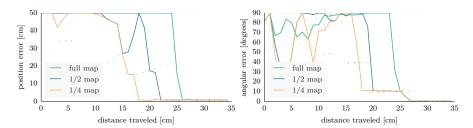
**Fig. 4** The error between the estimation by the localization algorithm and the ground truth, using Markov Localization, for different map sizes on linear trajectory. The solid lines show the median over 3 different trajectory parts, while the light dots show the individual parts.
