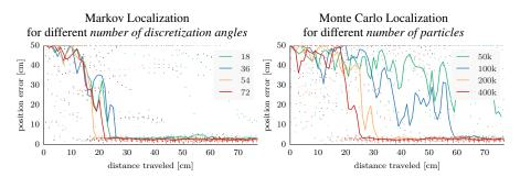
**Fig. 3** The error between the estimation by the localization algorithm and the ground truth on 10 segments from the first two trajectories. The solid lines show the median while the light dots show the individual trials.
