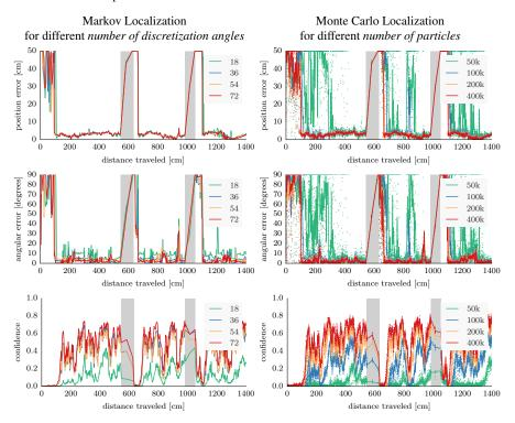
**Fig. 5** The error between the estimation by the localization algorithm and the ground truth, and the self confidence of the algorithm, on the run with kidnapping. For Monte Carlo Localization, the solid lines show the median over 10 trials, while the light dots show the individual trials. The gray areas show the time during the robot is being held in the air at the occasion of kidnapping.
