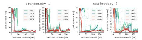
**Fig. 2** The error between the estimation by the localization algorithm and the ground truth on trajectory 1 and trajectory 2. For Monte Carlo Localization, the solid lines show the average over 10 trials, while the light dots show the individual trials.
