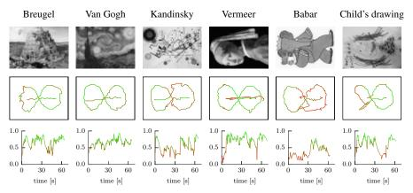
Fig. 6 The image, estimated trajectory and self confidence for different  $59 \times 42\,\mathrm{cm}$  grayscale patterns printed on A2 papers with a resolution of 1 pixel/cm. The robot is remotely controlled to draw a 8-shape figure, with similar motor commands for each image. Markov Localization with 36 discretization angles used. The color of the lines vary from red (confidence 0) to green (confidence 1). Trajectories are plotted starting from a confidence level of 0.2.
