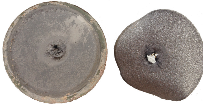
Figure 8.10 – Anode-supported cell after operation for 350 h under H 2 plus toluene, Ni mesh current collector used at the anode side after the test.
