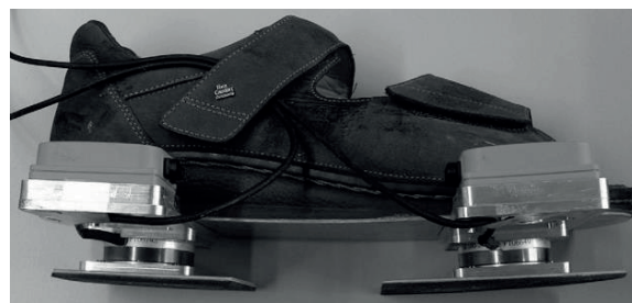
Figure 2-3 – Force sensing shoes from Schepers et al. [138] , same system used by Liedtke et al. [150] (©Schepers et al. [138])
