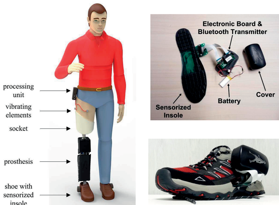
Figure 2-10 - Feedback system for amputees, a) system components at the thigh, prosthesis and shoe level, b) instrumented insole, c) insole cover placed laterally on the shoe (adapted from [220], [222])
