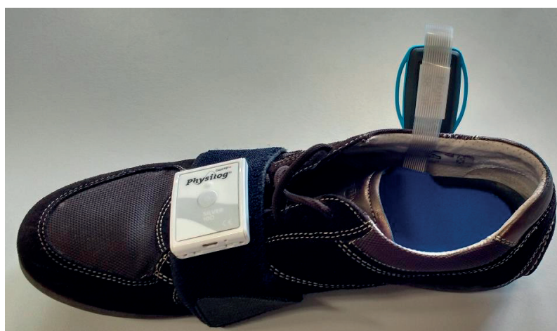
Figure 4-1 - Instrumented shoe system (right shoe). The Physilog® (GaitUp, CH) is placed on a strap looping around the shoe with Velcro® tape. The insole (in blue) is placed inside the shoe and linked to the Physilog® by a cable. Converting electronics are in the box with handles (lateral side of the shoe), connected to the strip stemming from the insole.
