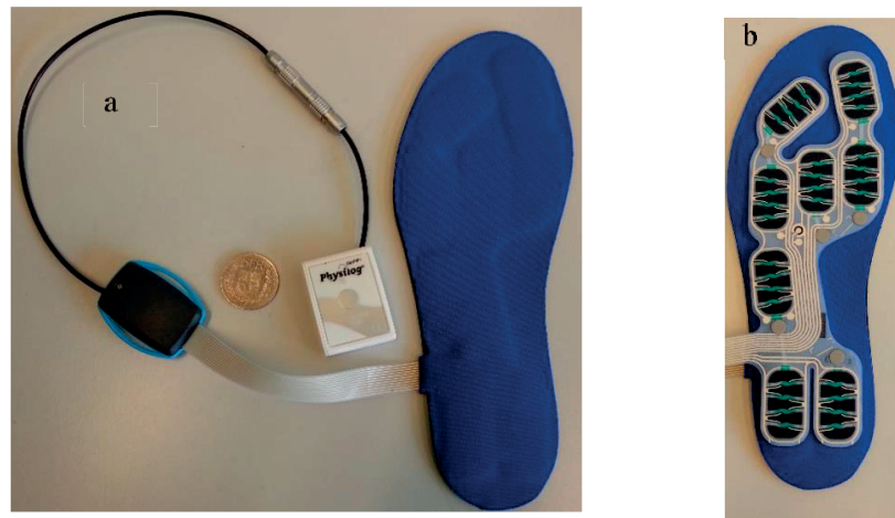
Figure 3-1 - (a) Instrumented shoes system. The Inertial Measurement Unit (IMU), force sensing insole and converting electronics (Gray box with blue handles). (b) Force sensing insole with 8 sensors.
