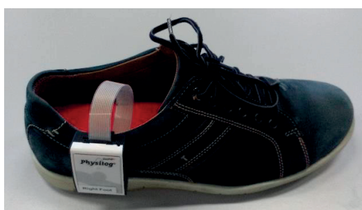
Figure 8-2 - Miniaturized instrumented shoe prototype with insole inserted in the shoe and inertial measurement unit clipped on the lateral side of the shoe. This system is also equipped with a Bluetooth data transmission chip
