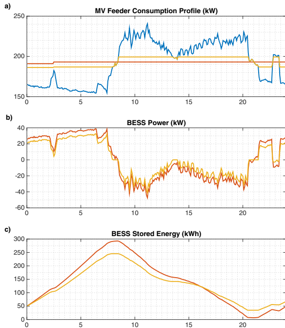
Figure 4. Comparison of a load leveling daily profile without BESS operation (blue), with BESS operating without ageing constraint (red) and with BESS operating with EOL constrained to 30 years (yellow).
