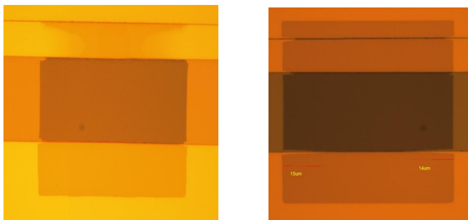
Figure 59: Broken SiO 2 bridges due to over etching of SiO 2 layer in BHF
