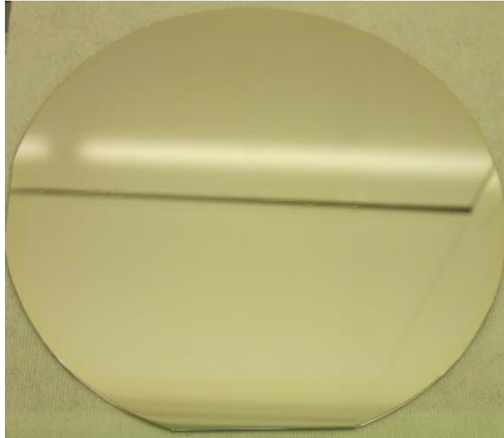
Figure 33: Appearance of silver color after Pt layer deposition
