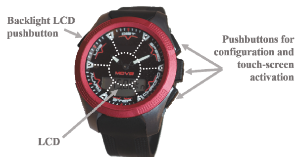
Fig. 1. The sport watch prototype and its user interface with the 7 sensitive zones of the touch-screen delimited by dashed white lines
