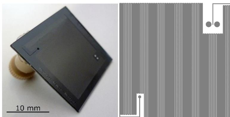
Figure 2 Left, microcolumn chip fabricated by MicroSens. Right, diagram of the original microcolumn geometry. Left image courtesy of Ulrike Lehmann.
