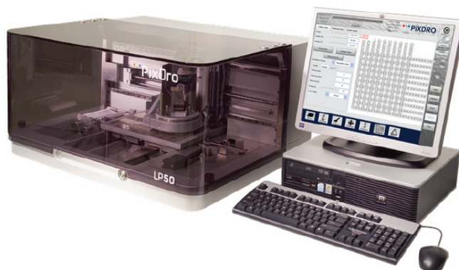
Figure 2.1: Image of the inkjet printer “PiXDRO LP50” [MB 2013], from Meyer Burger (Netherlands) B.V., used in this thesis to fabricate the interdigitated TCO/metal electrodes of our IBC-SHJ and tunnel -IBC-SHJ solar cells.
