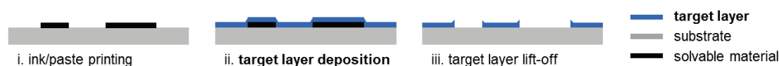
Figure 3.1: Schematic representation of the thin-film patterning method based on the use of a solvable material and target layer lift-off.
