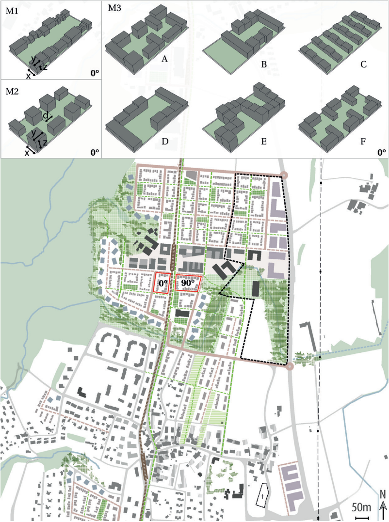
Figure 3.4 – Illustrative master plan of the LN-PDL study, with example plots (framed in red) on which the design variants created from M1 and M2 or the specific designs of M3 (top) could be located. Plan adapted from Urbaplan [2015].
