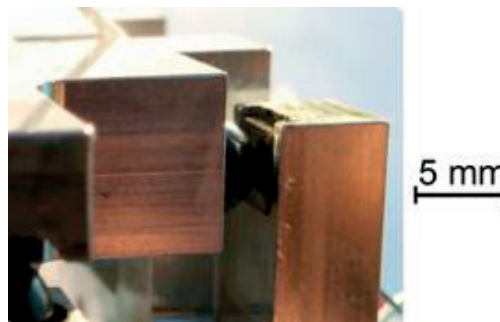
Figure 12.2.10: A contact sphere and contact flat of the three-body kinematic mount in contact.
