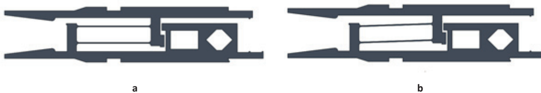
Figure 11.2: a) a single clip in neutral position b) a single clip in open position. It can be displaced further, up to a hard mechanical stop.
