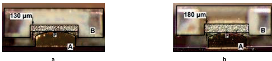
Figure 11.7: a) Application of solder at a contact point between two bodies causing an offset of 130 \mu\text{m} . b) Another contact point of the same assembly with an offset of 180 \mu\text{m} .
