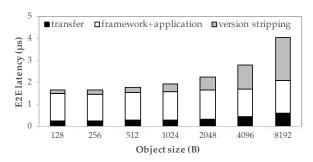
Figure 1: End-to-end remote object read latency using the per-cache-line-version software atomicity check mechanism on FaRM over soNUMA.
