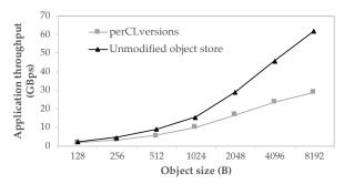
Figure 10: FaRM local reads throughput comparison.
