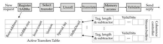
Figure 4: R2P2 microarchitecture.
