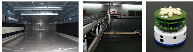
Fig. 5. The wind tunnel setup (left), the emulated aerial robot mounted on the traversing system (center), and a Khepera IV robot augmented with odor board and the anemometer board (right).
