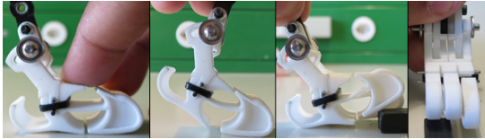
Fig. 2: Flexible foot prototype performing adaptation to different surfaces due to manually applied force.
