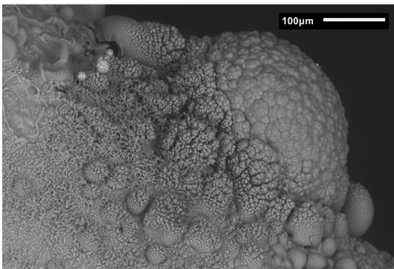
Fig. 8. SEM image of the surface (the hot zone) of octet specimen of group II after the tests. The swelled region correspond to an exuded bead after severe oxidation (a cross section of it can be seen also in the rectangle in Fig. 7).
