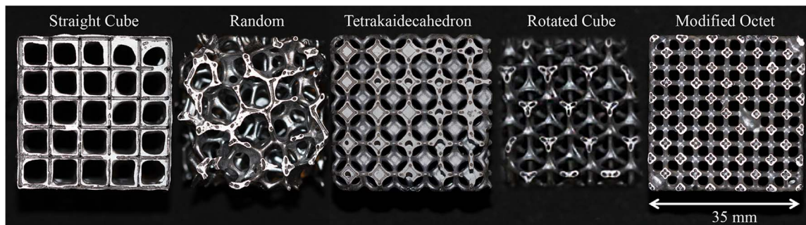
Fig. 1. Front view of the five SiSiC lattices produced by replica technique in this work.
