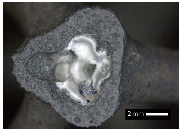
Fig. 4. Rotated cubic sample of group I after thermal oxidation. The cavities inside the struts oxidized in a lower oxygen partial pressure. That can result in formation of silica whiskers (white features). An exuded silicon alloy bead is also evident inside the strut.
