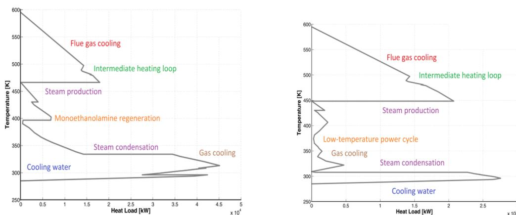
Figure 3: Balanced Grand Composite Curves for a steam network and monoethanolamine CO<sub>2</sub>-capture unit (left) and a combined steam cycle + low-temperature C<sub>2</sub>H<sub>6</sub>-C<sub>3</sub>H<sub>8</sub> power cycle (right)
