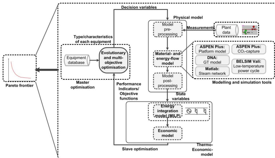
Figure 2: Framework methodology for the modelling and optimisation of the CO<sub>2</sub>-mitigation options
