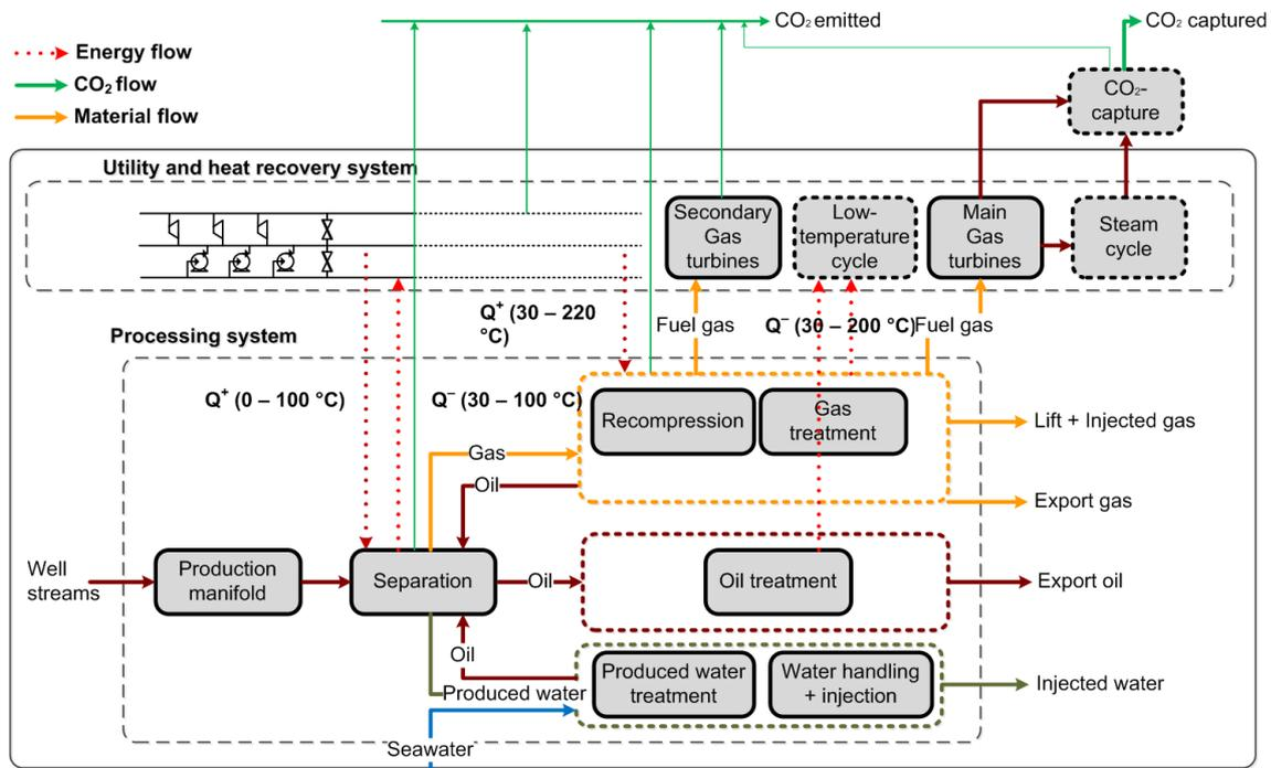
Figure 1: Process superstructure of CO<sub>2</sub>-mitigation options for oil and gas platforms
