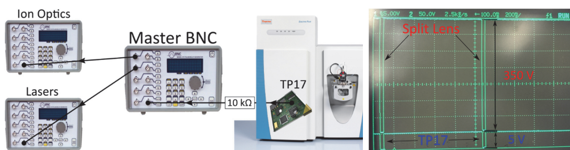
Figure 3.4. (Left panel) Schematic diagram of triggering the cold ion spectrometer by external pulses, taken from the test point TP 17 on the Ion Optic Supply RF board of the Exactive mass spectrometer. (Right panel) Snapshot of the oscilloscope display that shows a synchronization between the pulse voltage applied to the Split lens (from 0 to 350 V) and the TTL pulses at the test point TP 17.
