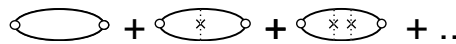
Figure 3: Ladder diagrams describing the conductivity within Born approximation. Solid lines and empty circles represent respectively G(\mathbf{p}, i\varepsilon_l) and j_x(\mathbf{p}) .
