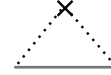
Figure 1: Wigwam diagrams which describe the self-energy within Born approximation. The solid line correspond to the dressed Green function, G , while the crosses indicate averaging over disorder [1, 2].
