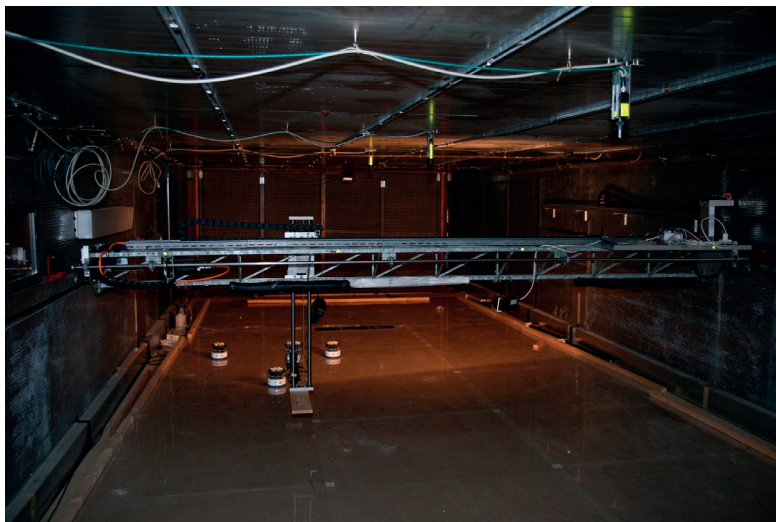
Figure 6.2 – Wind tunnel 3D traversing system, with Khepera IV robots in the background.
