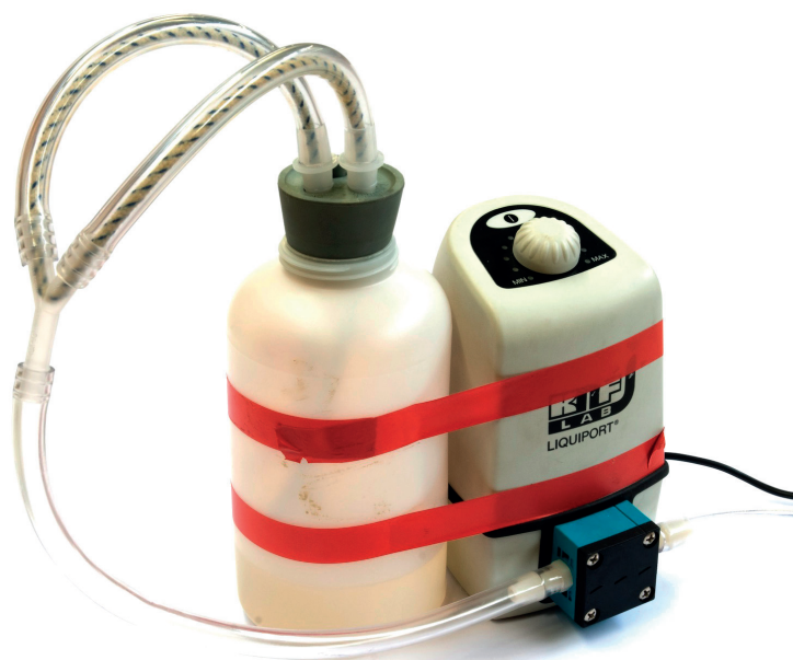
Figure 6.4 – Odour pump and ethanol reservoir.
