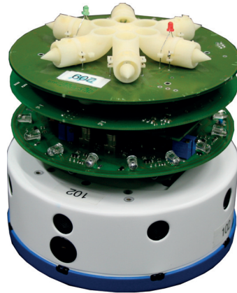
Figure 5.2 – Khepera IV robot equipped with the same sensor stack.
