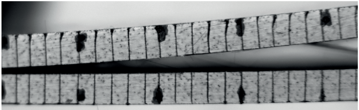
Figure 4.37: Mixed Mode \mu = 60\% , bridging tractions in the middle of the crack at \Delta a = 20mm
