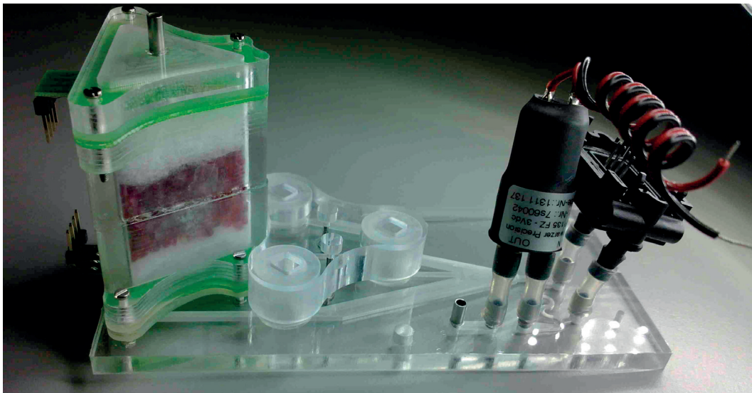
Figure 2.19 – Above is the metal oxide sensor platform. This design was specifically created to hold 3 of CEIT’s TO8 packaged sensors. However, because TO8 is an industry standard package, the device can be adapted to hold commercial sensors. It was also designed to be smaller and more integrated than the single sensor version.
