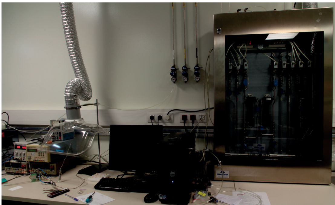
Figure 3.8 – One of the gas mixing systems at CEIT. The silver box contains all of the components in the pink box in Figure 3.7, with the exception of the gas tanks.
