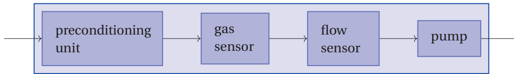
Figure 2.1 – Flow chart of the fluid path through the single sensor platform. For a flow chart of the components in the preconditioning unit see Figure 2.5.
