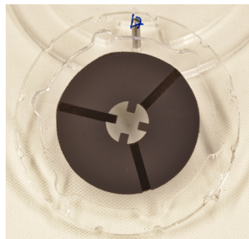
Figure 2: Printed membrane with 3 independent actuators for Rupert.
