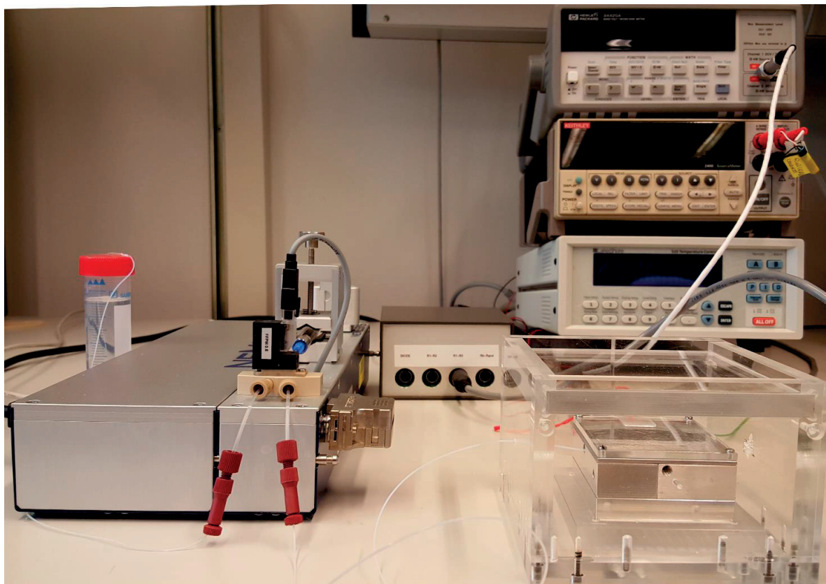
Figure 42 Photograph showing the nanocalorimetric platform and the necessary equipment. Acquisition equipment are on the right-hand side (from the top to the bottom): the nanovoltmeter, the sourcemeter and the temperature controller. On the back of the picture, the signal distribution box is visible. The syringe pump used for sample injection is on the left side. The foreground shows the nanocalorimetric platform, including the outer PMMA box surrounding the aluminium holder, which is used for additional insulation from external temperature fluctuations.
