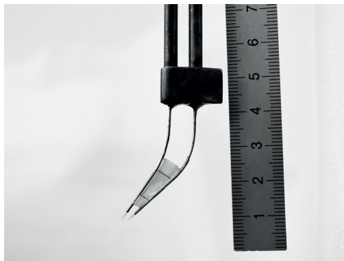
Figure 3.12 – The tips of the fiber optical probe. The optical fibers are protected in thin metallic tubes until the last few millimeters. The sapphire prisms are the light tips at the end of the metallic tubes. The probe is oriented for a flow from left to right. The measuring tape is in centimeters
