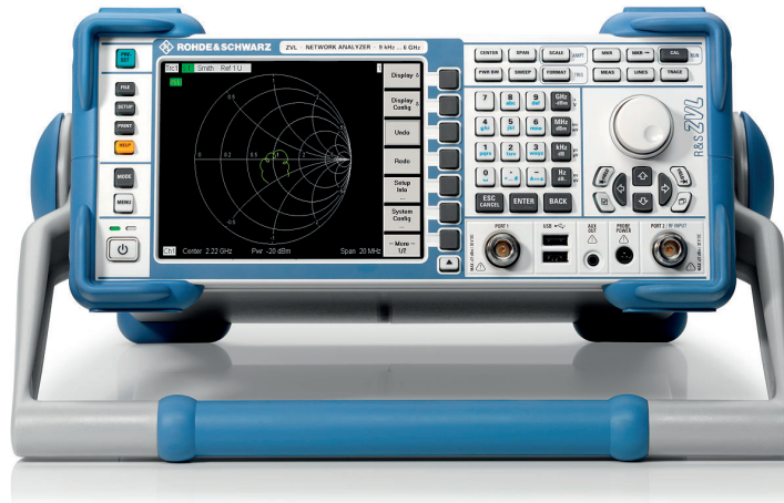
Figure 3.14: Rohde & Schwarz ZVL 6 vector network analyzer.
