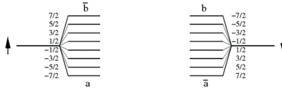
Figure 2.6: Lowest nuclear-electronic states of the electronic doublet split by the hyperfine interaction. After M. Schechter and P. C. E. Stamp [21].
