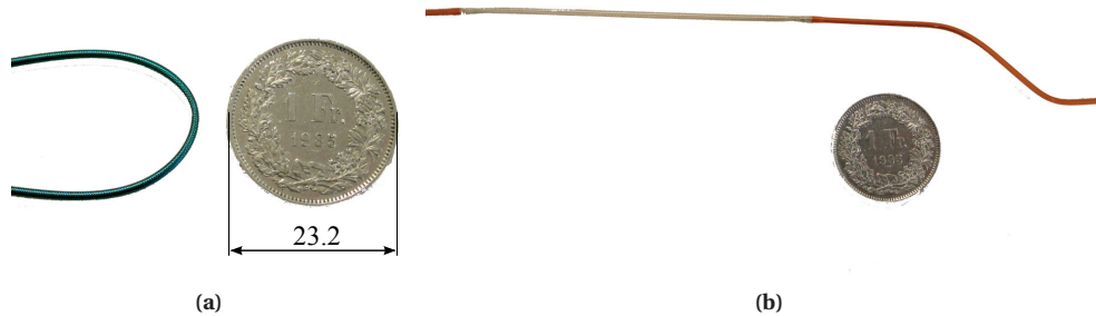
Figure 2.10: Composite polyimide tubes: (a) pipe with reinforcement coil and outer surface made of Pebax ® ; (b) pipe with a PTFE transition plus shaped polyimide section. Dimensions expressed in mm.
