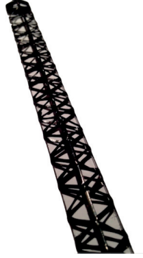
Figure 2.6: A view of a primitive ALICE ITS Upgrade module made of M55J CFRP. From [4].
