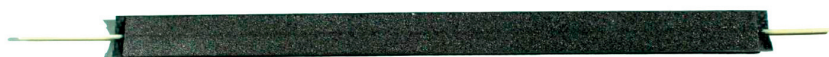
Figure 2.5: Carbon foam and PEEK cooling channel used in a primitive ALICE ITS Upgrade module, 290 x 15 mm in size, [4].
