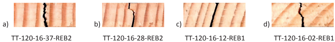
Fig. 4.16: Different failure types observed in specimens: a) Earlywood failure b) Earlywood-border failure c) Growth ring border failure d) Crossing growth ring failure. Vertical dimension is 4mm (specimen width). Load is applied in horizontal direction.
