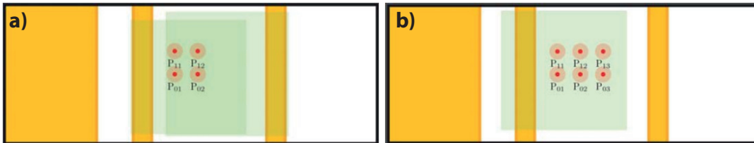
Figure 5.14: Various spatial points representing the incoming THz beamwidth distributed along a) graphene stack and b) single layer graphene surfaces employed to study the uniformity of the samples.
