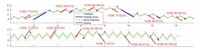
Figure 2: Footstep plan using DLQR (top) and projecting (bottom) controllers. The DLQR reacts to intermittent pushes only at the end of the phase while the projecting controller updates inputs continuously. Note the percentages that show force application timing.
