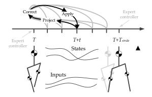
**Figure 1:** The overall idea of time-projection where the current state is mapped back in time to the beginning of the phase. It is then given to an expert controller whose output is used in the current time-step to stabilize the system online.
