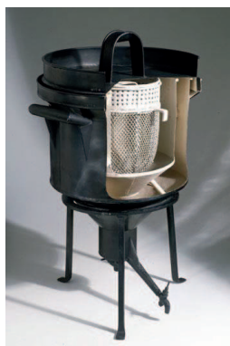
(a) Calorimeter of Lavoisier and Laplace (from Science Museum, London [Ice calorimeter])
