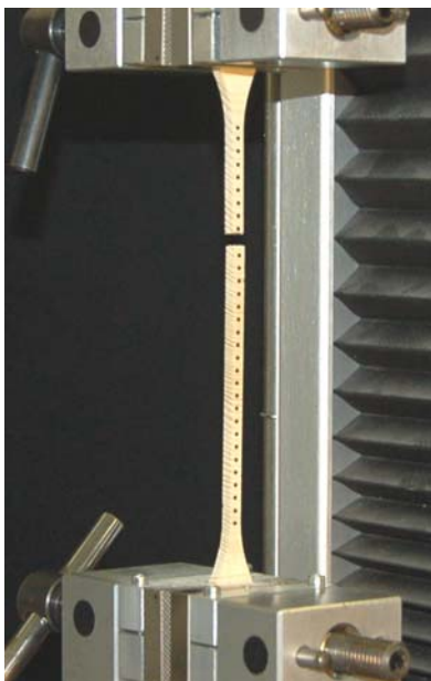
Figure 2: Specimen of 120 mm nominal length with applied dots inside machine grips.
