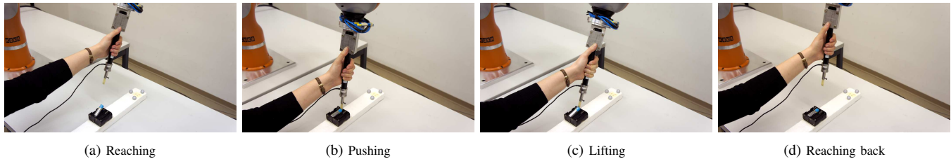
Fig. 12: Atomic actions in performing the task. The task typically consists of reaching for the battery stand, applying a force that tensions the spring inside the support (pushing), taking out the battery (lifting), and reaching away
