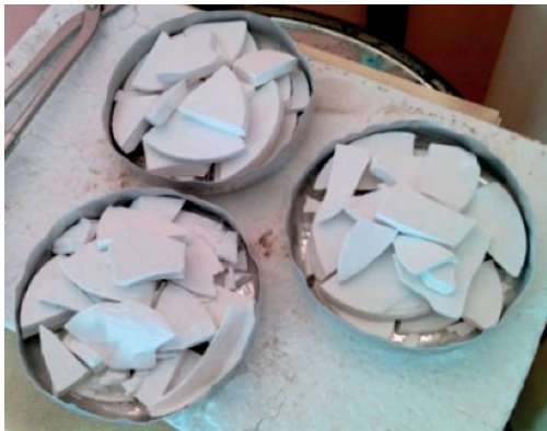
(a) Homogenized powder pellets in Pt crucibles before firing
