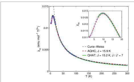
Figure 2. Magnetic susceptibility  $\chi_{\rm m}(T)$  of Ti-yavapaiite. The experimental data recorded at 1000 Oe is plotted with blue circles, while the fits to the Curie–Weiss law, the AQHC, and the QHAT are indicated by black dashed, red dashed, and green solid lines, respectively. The latter is only plotted down to 8  $K \simeq 0.8T_p$  due to the divergence of the [5,5] Padé approximant below this temperature. The inset shows a magnified region around the low temperature peak.
