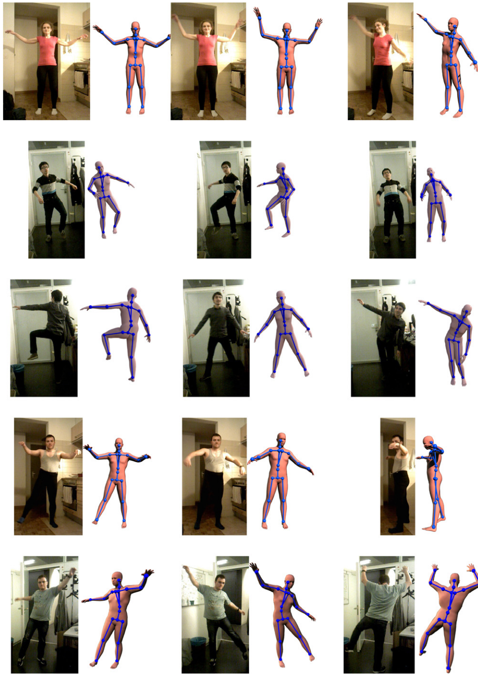
Fig. 9. The proposed framework is able to track bodies and estimate their parametric body model from a depth sequence. In each row of the figure, we report three examples of a sequence corresponding to one of the evaluated subjects ( S_1 , S_2 , S_3 , S_4 , and S_4 , respectively). For each example, we show the input RGB frames, the posed body and its corresponding skeleton.
