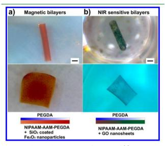
**Figure 1.** Tubular and rectangular configurations of (a) a magnetically responsive hydrogel nanocomposite containing silica coated iron oxide nanoparticles and (b) a NIR light-responsive hydrogel containing GO nanoparticles. Scale bar is 500  $\mu$ m.
