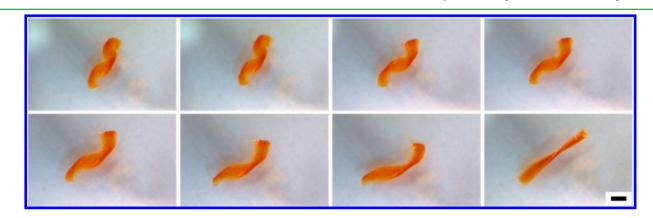
**Figure 5.** Temperature-dependent folding of a magnetic hydrogel ribbon. The temperature range is 20 °C, from (upper left) 25 °C to (lower right) 45 °C. Scale bar is 0.5 mm.
