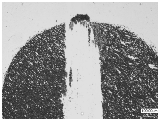
Figure S6. Optical micrograph of a micro-scratched tissue section after several repetitions of an SECM line scan using a conventional Pt ME enclosed in an insulating glass sheath.
