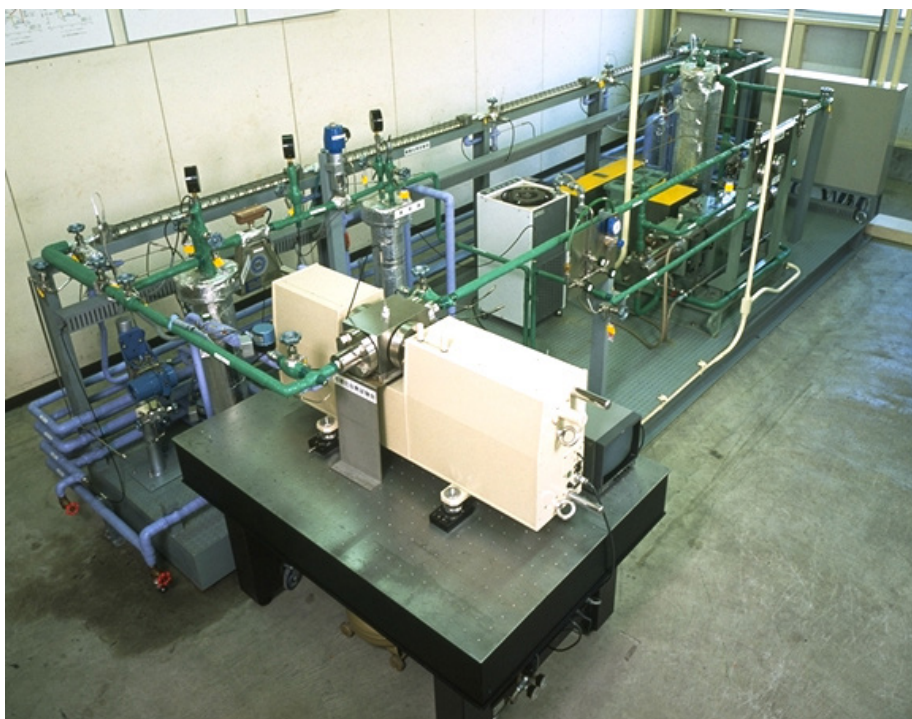
Figure 5. Basic experiment loop for CO 2 heat pump. Heating capacity 4 kW, installed in 1996.
