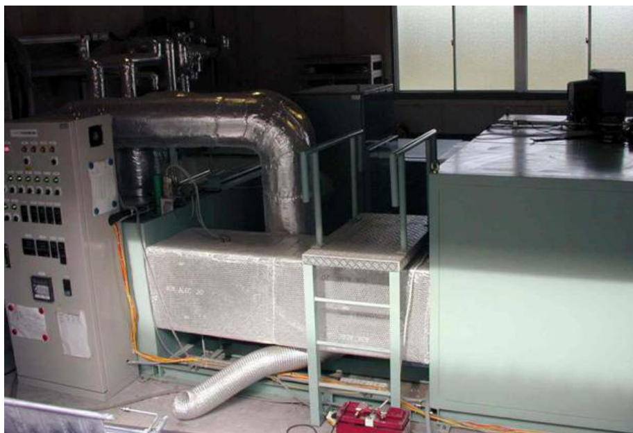
Figure 6. Test chamber for prototype of CO 2 heat pump water heater. Heating/cooling capacity 5 kW, installed in 1999
