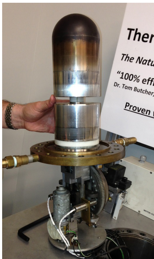
Figure 4. Pictures of BVE's mechanically-driven 4kW VHP prototype
